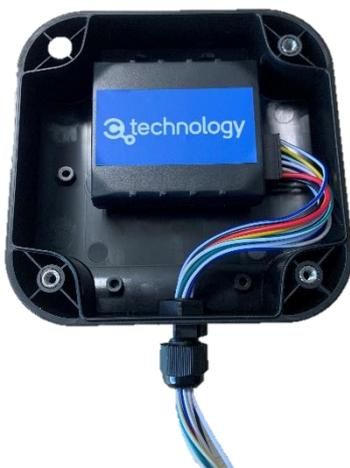
In the first step, the c.technology-computer should be placed in the housing, if desired, and the signal cables should be plugged in. In the second step, the cables are connected to the individual components of the boat.
